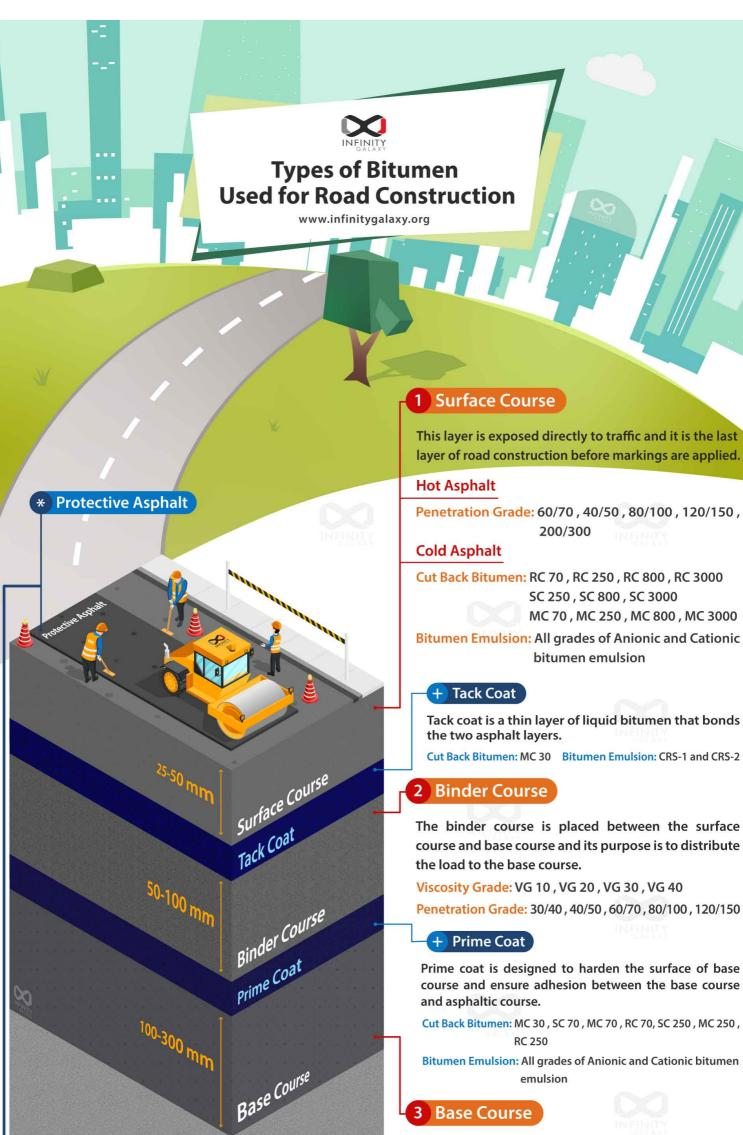
Tack coat is a thin layer of liquid bitumen that bonds
